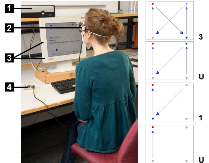
Figure 6. Experimental setup consisting of a desktop computer running the game (1), the Goggles (2), a flat screen with red dots used for calibration (3) and the Pocket (4). The screenshots on the right show the sequence of eye movements and the generated event symbols for gesture 3U1U (from top to bottom). The red dot denotes the start of the gesture and the blue dot its end point. Blue arrows indicate the order and the direction of each expected eye movement and are masked out after having been successfully performed.
