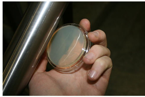
Fig. 3 Samples were taken from the bus pole on the agar plate to evaluate the number of colony forming units (CFU)
