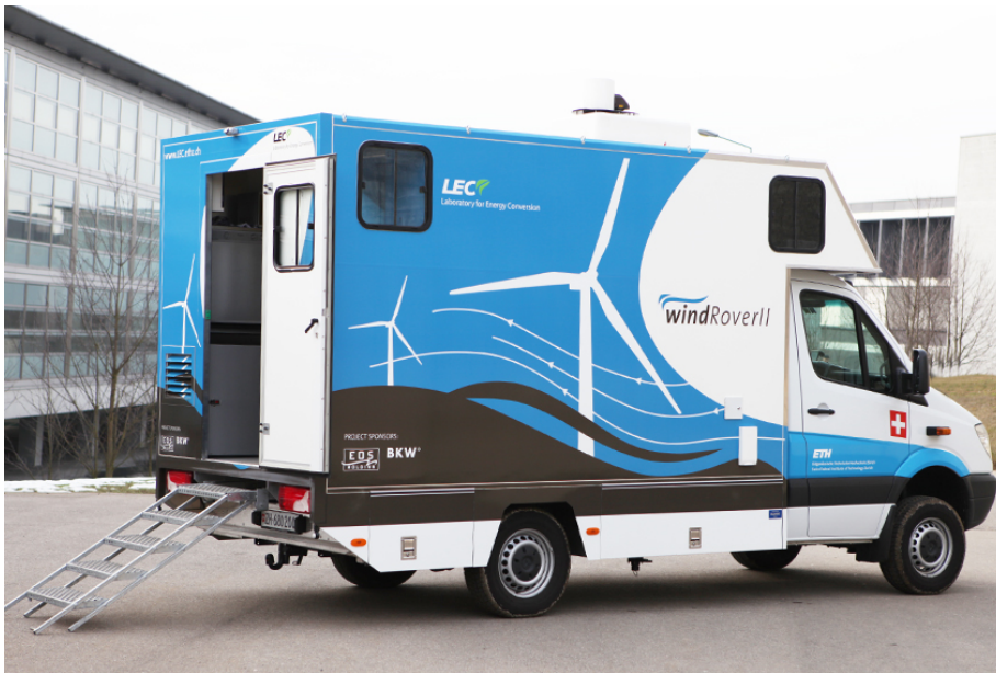
Figure 2.2: WindRoverII, mobile laboratory equipped with 3D scanning LiDAR system.
