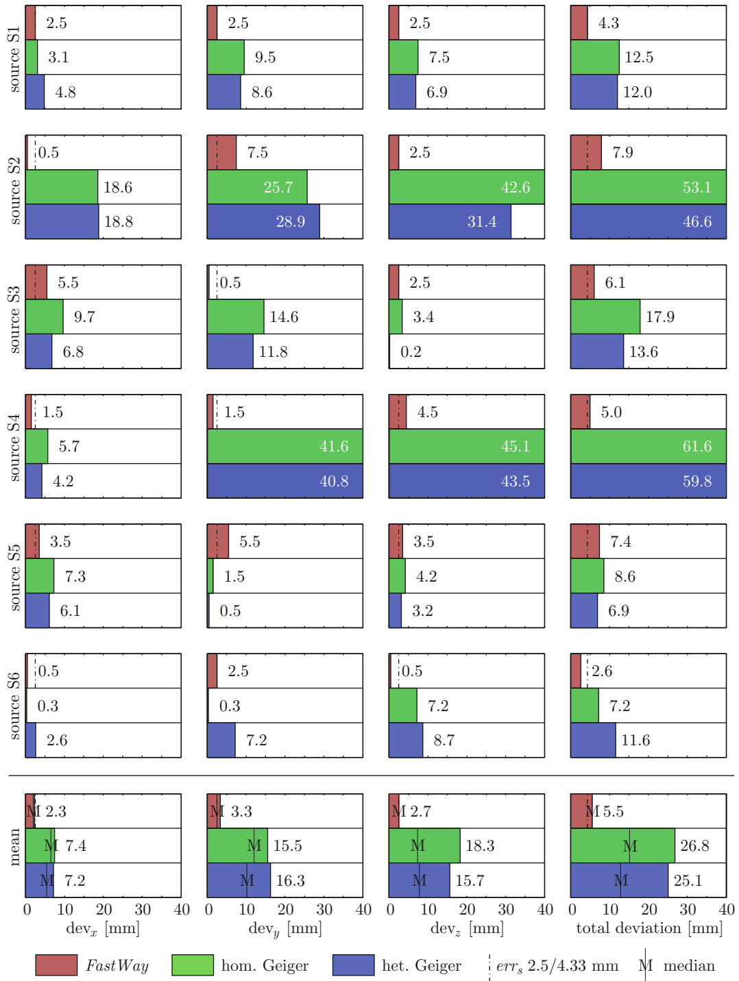
Fig. 5.12: Visualization of the deviation between the estimated and actual source locations. In the last row the mean (colored bar) and the median of the deviations are visualized for all six sources. The parameter err_s is marked in the bar representing the FastWay solution (2.5 mm in each direction; 4.33 mm in total)
