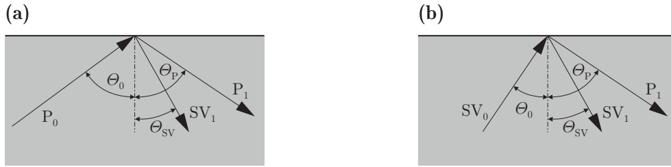
Fig. 2.3: Reflection and refraction at a free boundary of (a) a p-wave and (b) an sv-wave (adapted from [22])
