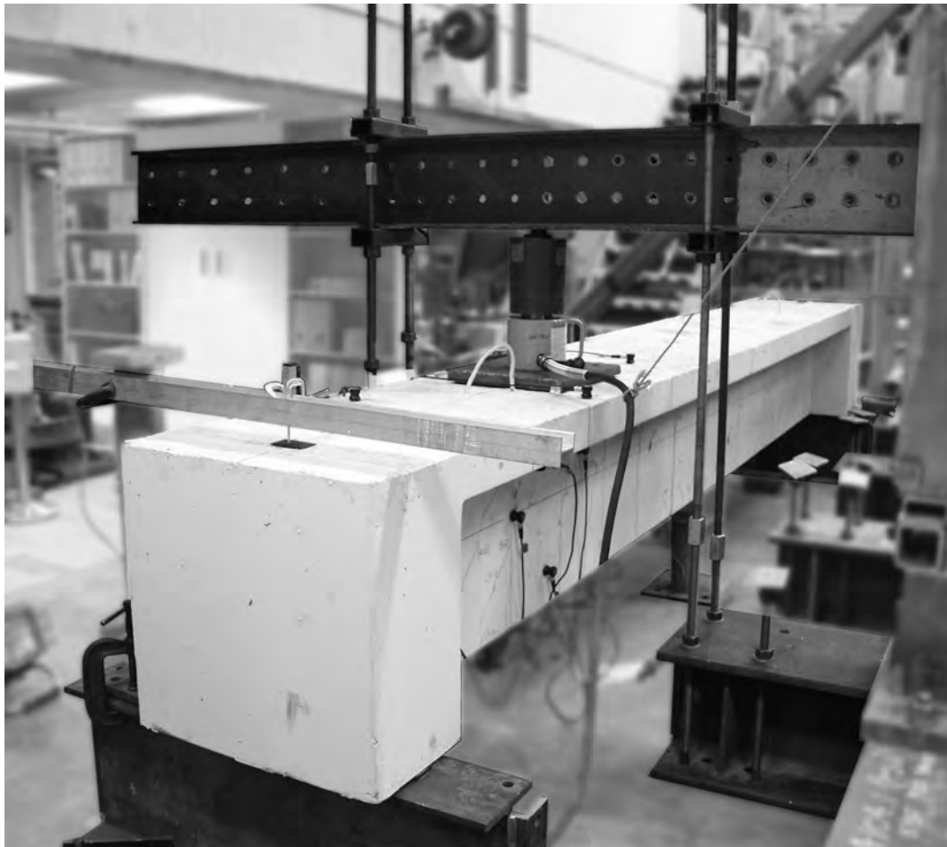
Fig. 7.55: Test setup of shear test SW II.
