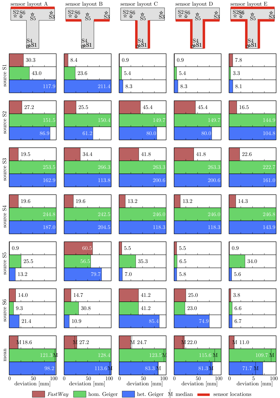
Fig. 5.18: Visualization of the deviation between the estimated and actual source locations. In the last row the mean (colored bar) and median of the deviations for all six sources are visualized.
