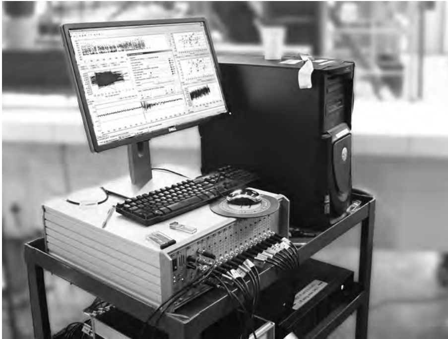
Fig. 7.5: The AMSY-5 data acquisition setup consisting of a M16-2 master unit, PC tower, keyboard, mouse, and monitor
