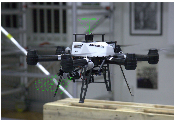
Fig. 11 The AscTec Neo hexacopter MAV is depicted, with the fields of view of the stereo camera pair and the upward facing camera visualized in green (Color figure online)
