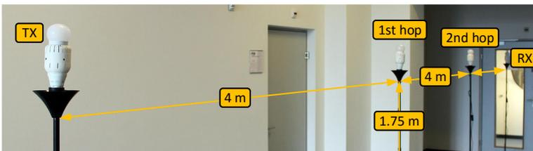
Figure 4.11: Deployed light bulb multi-hop testbed. The light bulbs are placed in floor lamps at 1.75 m above the floor level. The torchieres are setup in a line with a pitch of 4 m between each light bulb. A light bulb sensors orientation towards the next light bulb is chosen with a 45° offset (the middle between two sensors).
