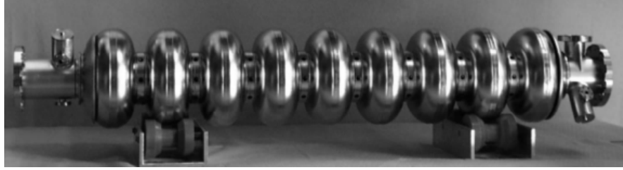
Figure 1.10: Superconducting 1.3 GHz 9-cell cavities designed for the TESLA Test Facility and used for FLASH in Hamburg, Germany. Reprinted from [12].
