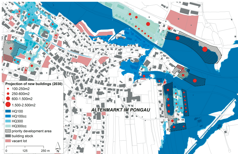
Figure 1: Current flood hazard exposure of buildings and expected future settlement development (until the year 2030) in an alpine floodplain (case study Altenmarkt im Pongau). (Source: IRUB)
