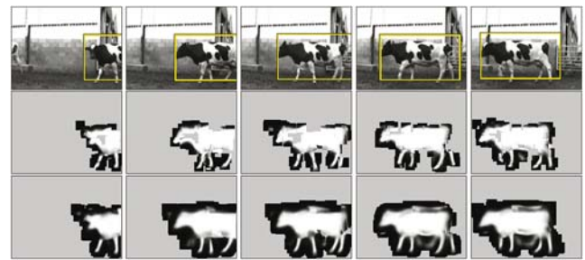
Fig. 20 Example detections and automatically generated segmentations from one cow sequence. ( middle row ) segmentations obtained from the initial hypotheses; ( bottom row ) segmentations from refined hypotheses (with additional features sampled in a uniform grid)
