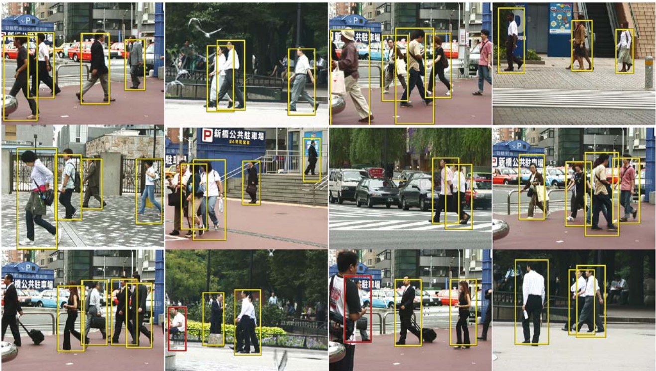
Fig. 22 (Color online) Example detections of our approach on difficult crowded scenes from the TUD Pedestrian test set (at the EER). Correct detections are shown in yellow, false positives in red
