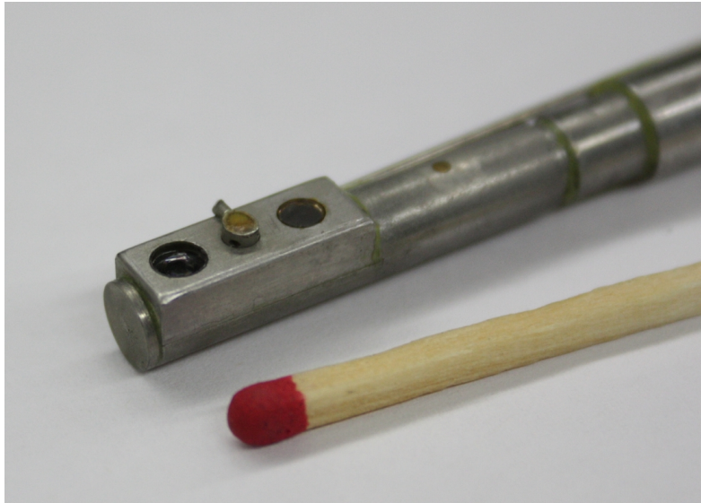
Figure 3-2: The optical backscatter probe tip.
