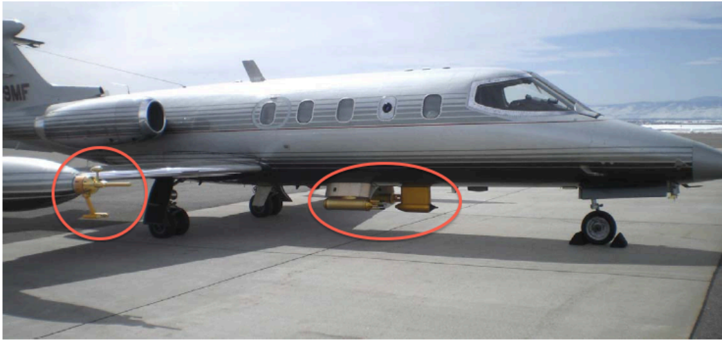
Figure 1–15: Optical probes used in atmospheric research mounted on aircraft's fuselage and wing [56].
