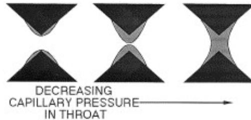
Figure 2.19.: Schematic representation of snap-off in a pore. (Rossen 2000)
