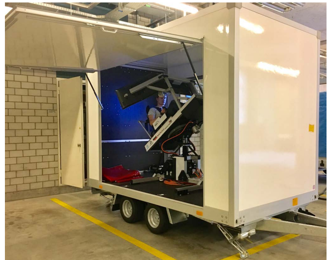
Fig. 8. ibex is mounted in a custom trailer with side walls that can be folded out.
