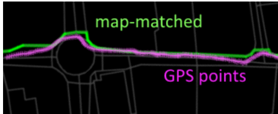
Figure 10.1: Map-matching walk stages: GPS points on roundabout, weighting ensures that side-walk and crossing are chosen
