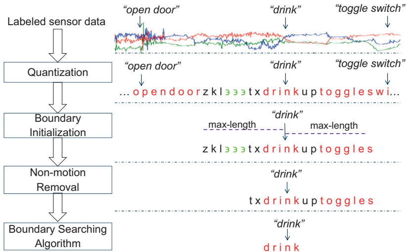
Figure 7.1: Data processing flow of the proposed boundary fixing approach. An example is shown on the right. Three annotated gestures "open door", "drink", and "toggle switch" with their one-time point annotations indicated as black arrows are given in the training data. In this example, the maximum length of "drink" gesture is given and it is used to initialize the boundaries of the "drink" gesture. \exists represents non-motion symbols.
