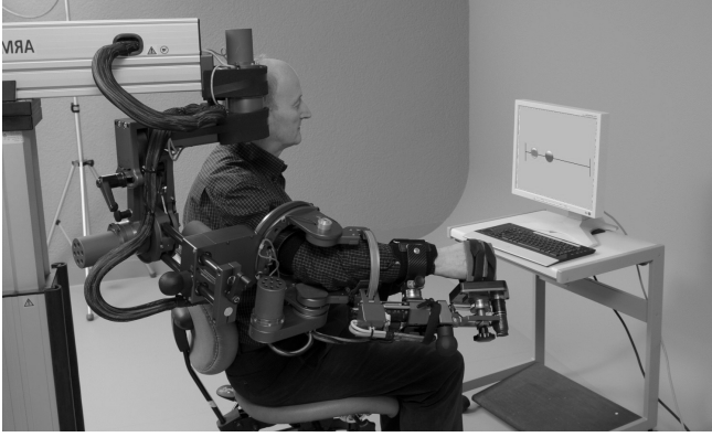
Fig. 3. Subject using the ARMin arm robot. The visual display is used to present task visualization.
