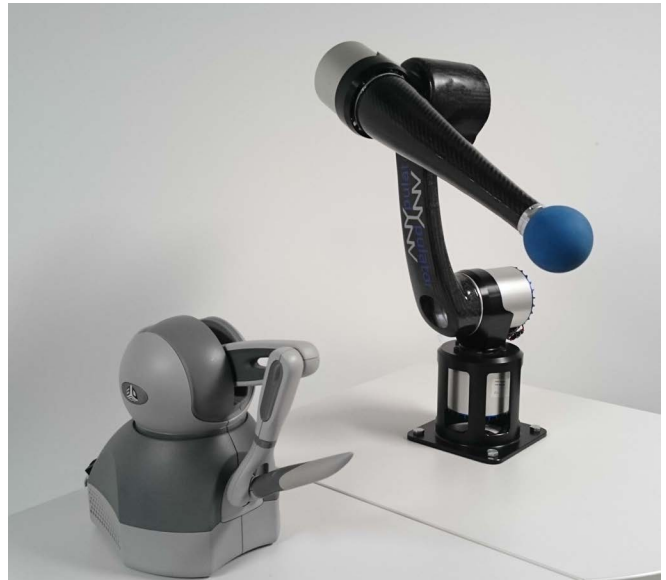
Fig. 1. Geomagic Touch is used for haptic teleoperation of ANYpulator
