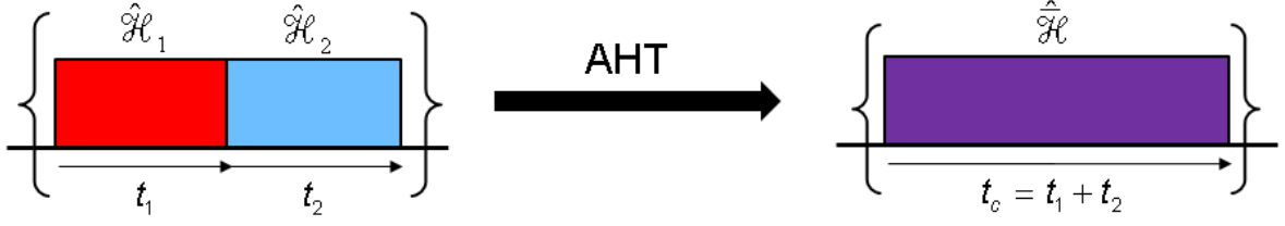
Figure 2.2 Schematic representation of the replacement of a time-dependent Hamiltonian \hat{\mathcal{H}}(t) by an average Hamiltonian \hat{\mathcal{H}} .
