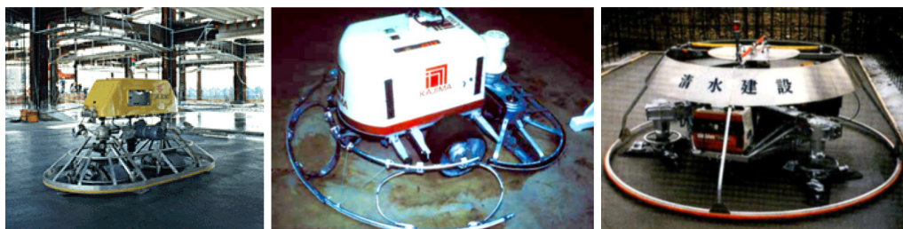
Figure 9. Concrete finishing robots. (left) SurfRobo by Takenaka Cooperation; (middle) Mark II , also known as Kote-King , by Kajima Corporation; (right) FLATKN by Shimizu Corporation.
