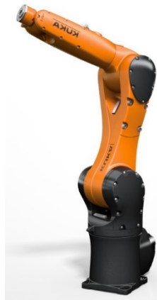
Figure 7. The KR 6 R900 sixx is part of the KUKA AGILUS family, which was introduced in 2012. Its kinematic design is noticeably similar to the robot models introduced in the 1970s, shown in Figure 6.
