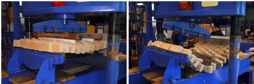
Figure 83. Bending Test: (left) Element before load; (right) failure of element.
