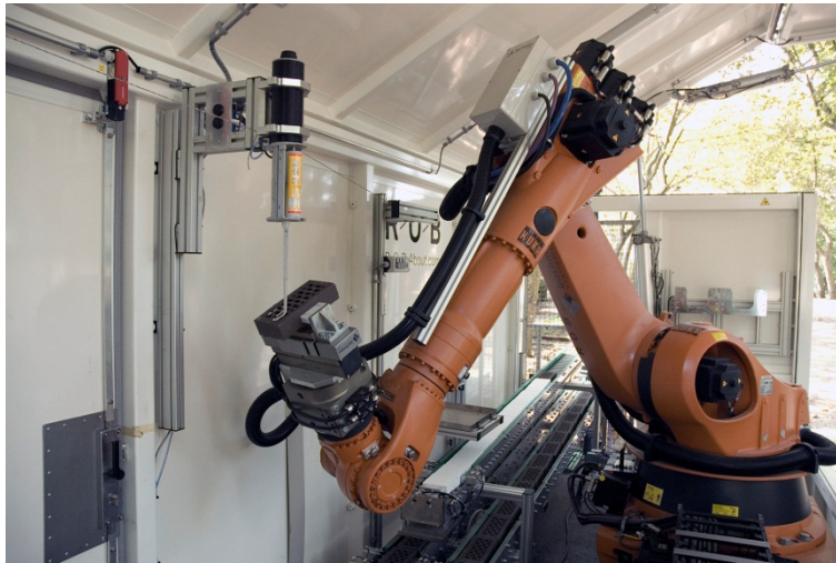
Figure 60. ROB Unit: showing parallel gripper and dispenser for structural adhesive.
