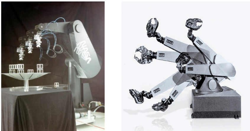
Figure 6. (left) Puma Robotic Arm, a further developed version of Scheinman's Stanford Arm by Unimation and General Motors, which was launched commercially in 1979; (right) KUKA FAMULUS .
