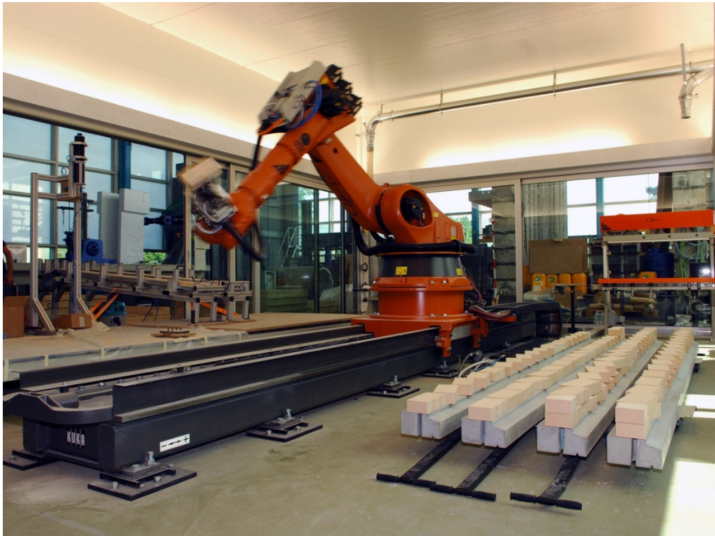
Figure 42. Experiment 2: Robotic assembly of elements for the non-standard brickwork façade of the Gantenbein winery (see Section 4.5.5).
