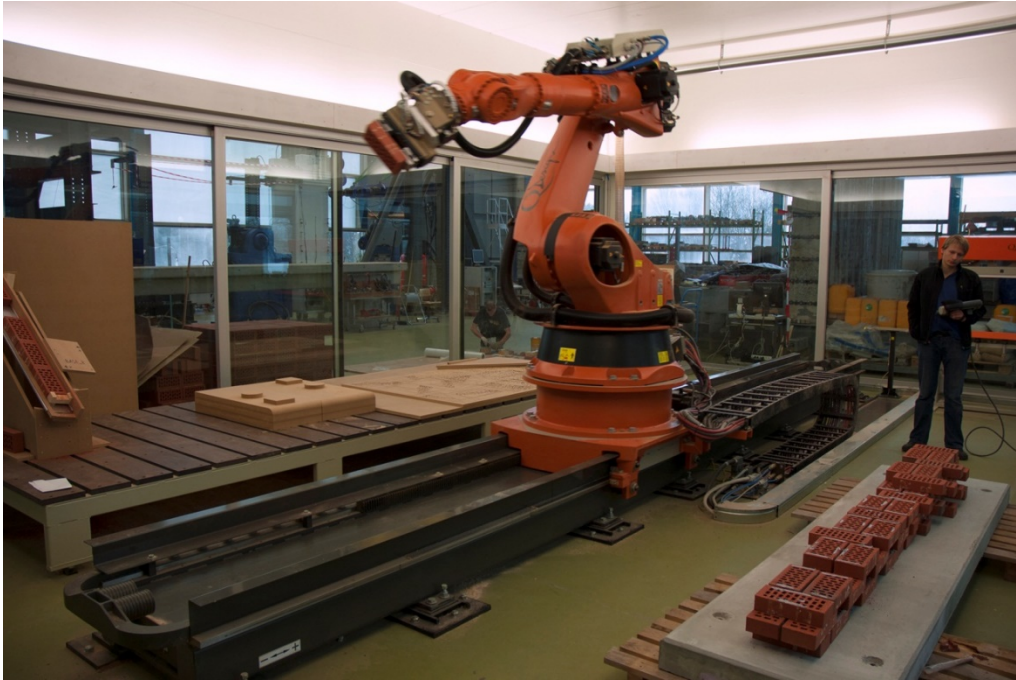
Figure 30. Experiment 1: Robotic assembly process (see Section 4.4.1).
