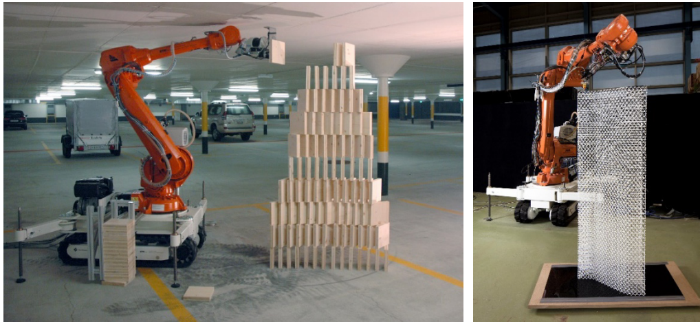
Figure 13. DimRob performing different fabrication processes: (left) assembling discrete wooden elements; (right) Prototypical mesh-mould process extruding thermoplastic polymers.
