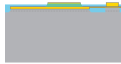
Figure 3.3 (cont.) (f) Collector metal stack deposition ( (f.1) side view, (f.2) top view ) (g) Isolation mesa etching ( (g.1) side view, (g.2) side view ) (h) Teflon planarization ( (h.1) top view, (h.2) side view )
