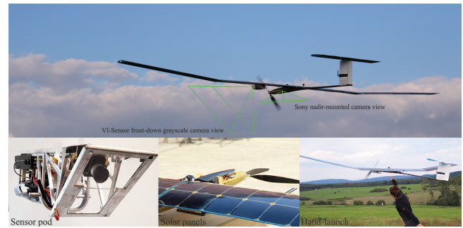
Fig. 10: The AtlantikSolar UAV with the sensor pod attached to its wings and further photos of the sensor pod, the solar cells and an instant of the hand-launching.
