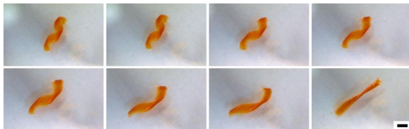
Figure 6.10. Temperature dependent folding of a magnetic hydrogel ribbon. The gradient of temperature was set to 20°C, from 25°C (upper left image) to 45°C (lower right). Scale bar is 0.5 mm.
