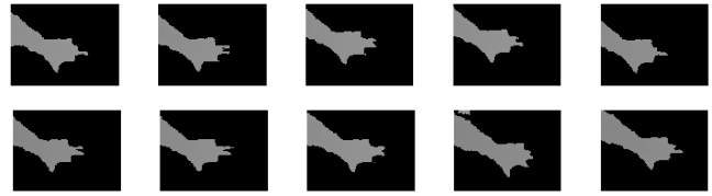
Figure 16: Ten consecutive frames of Kinect depth data similar to Figure 4 but with the filter. The arm and hand are reliably detected, fingers are not.
