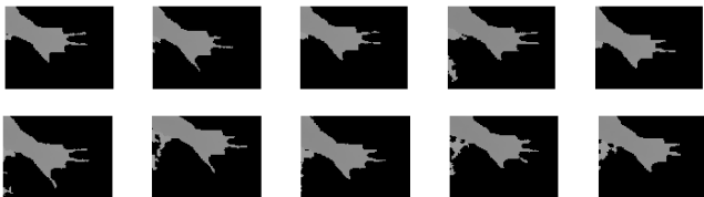
Figure 5: Ten consecutive frames of PixelSense depth data based on Figure 3 (cropped to only show hands). A stretched out hand can be seen from above. The fingers are irregularly detected.
