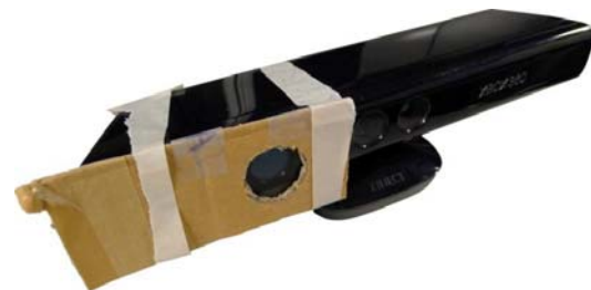
Figure 10: A linear polarization filter is used to attenuate the Kinect's IR-light. A piece of cardboard holds it in place.
