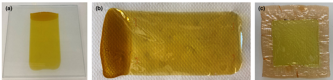
Figure 2. a) 19 \mu\text{m} m -PBI membrane on glass, b) free-standing 14 \mu\text{m} m -PBI membrane, and c) 13 \mu\text{m} Ethyl63 membrane after 200 cycles at 200 \text{ mA cm}^{-2} .
