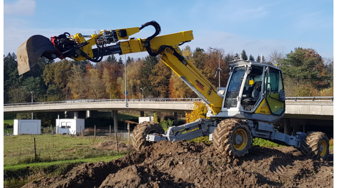
Fig. 1. Menzi Muck M545, a 12t hydraulic walking excavator.
