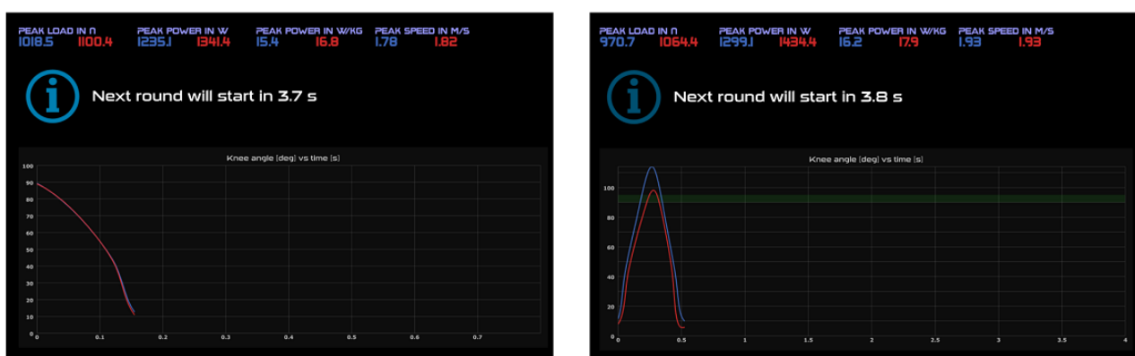
Figure 4. Left: Display of the visual feedback during the Real Power test on the soft robot. Blue and red lines, the knee joint flexion angle of the left and right leg versus time. Right: Display of the visual feedback during the Reactive Power test on the soft robot (source: Daniel Fitze, Dynamic Devices AG).
