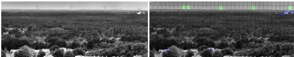
Figure 4.11: Figure showing algorithm results. Wind mills are mistakenly included as smoke
