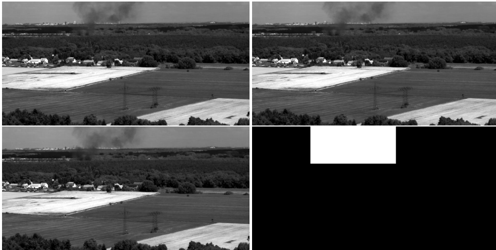
Figure 2.4: A triplet of images with its ground truth. First, second and third triplet images are shown at Top left, top right, bottom left respectively. Bottom right image shows the ground truth where white represents smoke region
