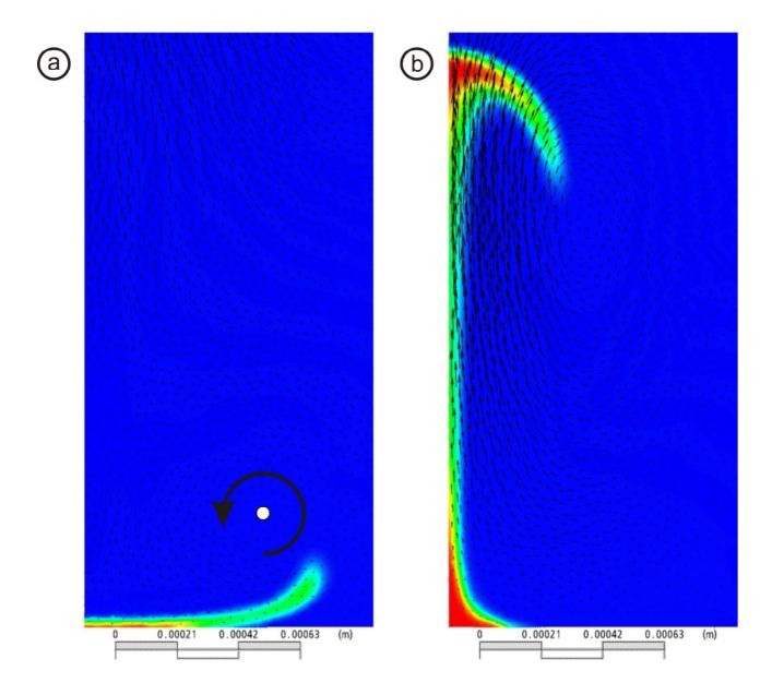
Fig. 4 Temporal progression of expanding aerosols generated by NIR-ns-LA using helium as aerosol carrier within a time interval of 63 ms
