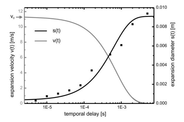
Fig. 8 Temporal progression of expanding aerosols generated by NIR-fs-LA using helium as aerosol carrier within a time interval of 63 ms
