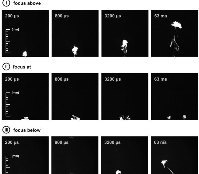
Fig. 6 Expansion study of an aerosol generated by NIR-fs-LA using argon for time delays up to 10 ms. Please note, that the image acquired for 10 ms does not show the entire aerosol but only the tailing part. The red sphere shown in the first image indicates the position of the laser focus
