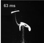
Temporal progression of expanding aerosols generated by NIR-fs-LA using argon as Fig. 5 aerosol carrier within a time interval of 63 ms
