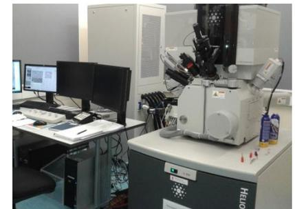
FEI Helios dual beam FIB with EDAX-EBSD
