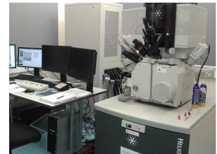
FEI Helios dual beam FIB
