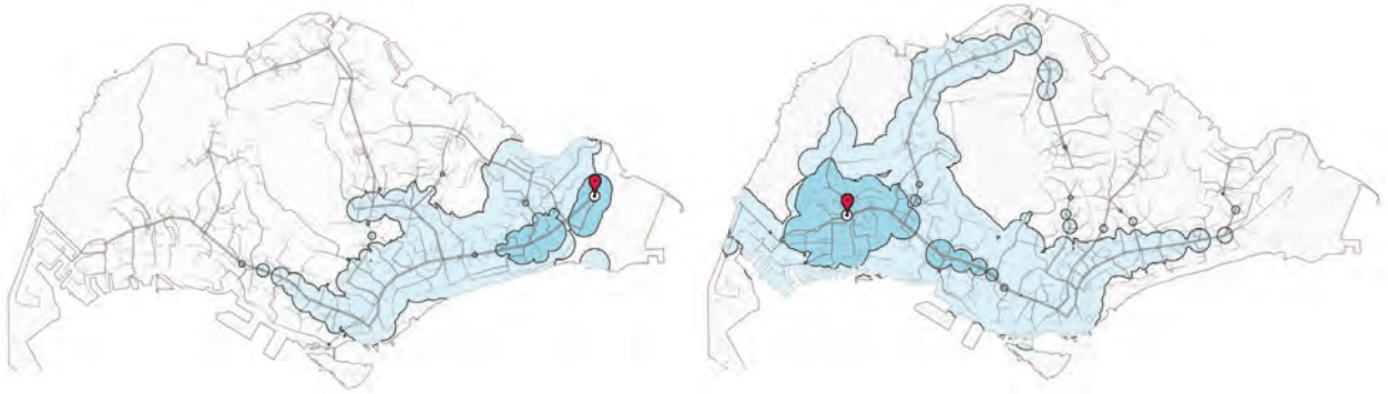
Fig. 06 The isochrone map views present spatial-reachability regions from 8 A.M. at origin (red icons) Changi Airport (left) and Boon Lay (right), by contour lines and areas over the geographical map. Dark blue and light blue indicate [0, 30] and (30, 60] minutes, respectively.
