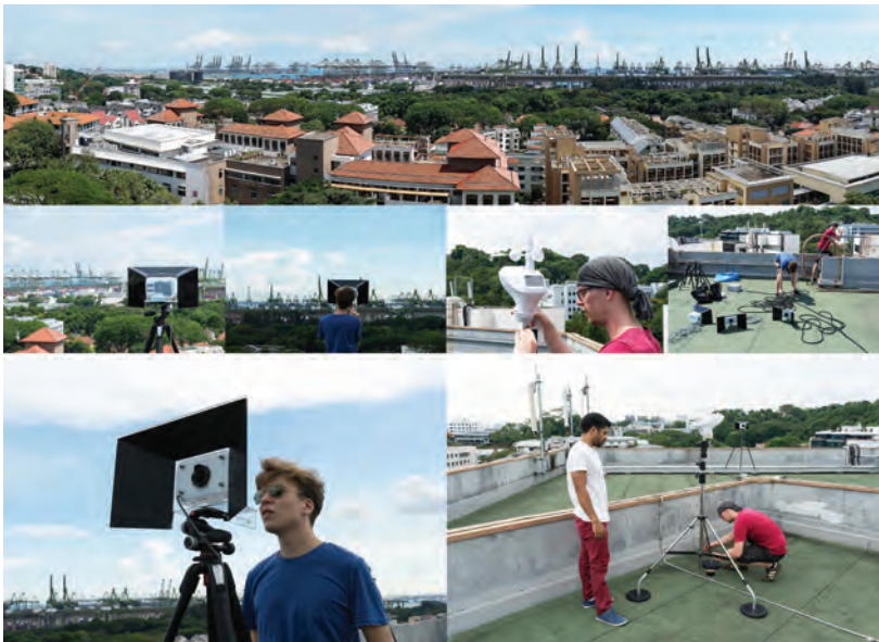
Fig. O3 Final setup of weather time lapse cameras and weather station on the rooftop of the I-Cube building at NUS campus
