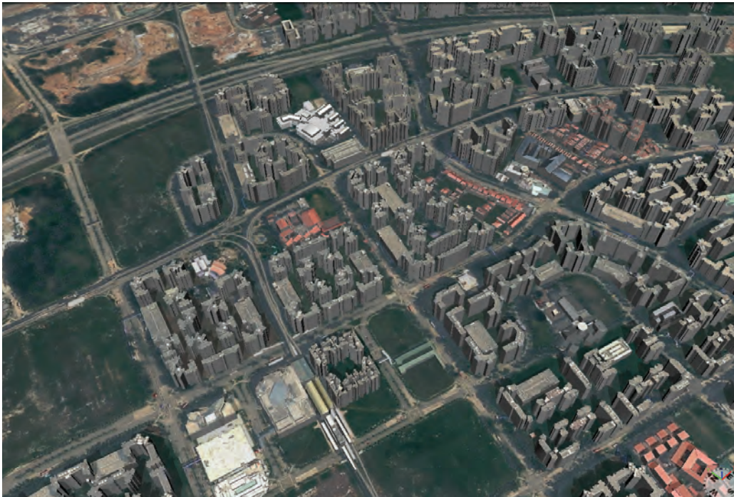
Fig. 01 Partially textured 3D city model of Punggol, Singapore. The model was derived from a WorldView-2 stereo-model by using CyberCity Modeler.
